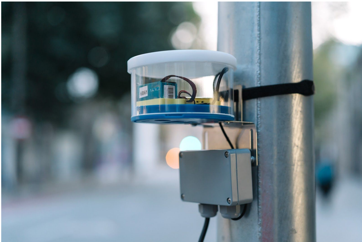
Figure 17. 3D-printed enclosure for SCK2.1 with Plantower PMS5003
