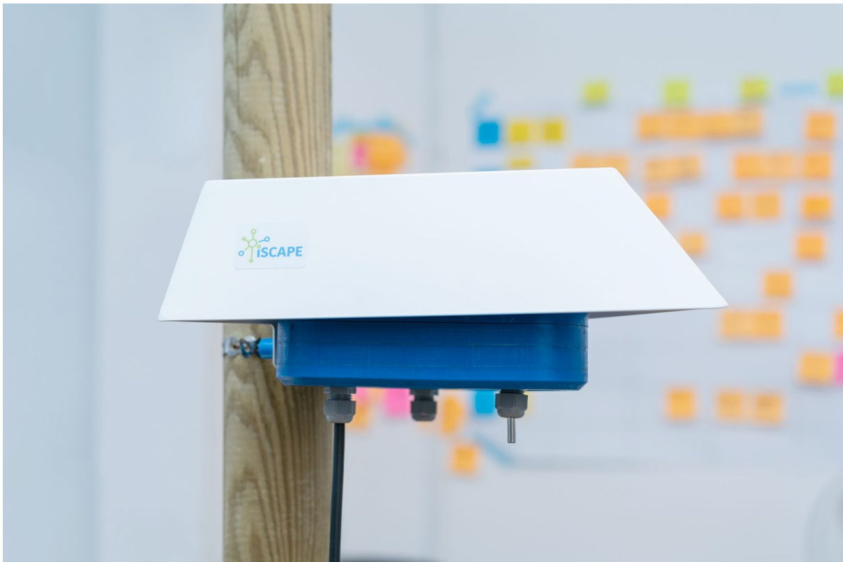
Figure 19. Cover and external temperature sensor
